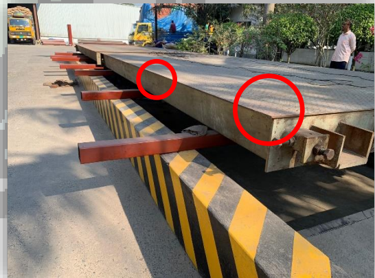
Picture: Disadvantage of welding the platform of other scales
