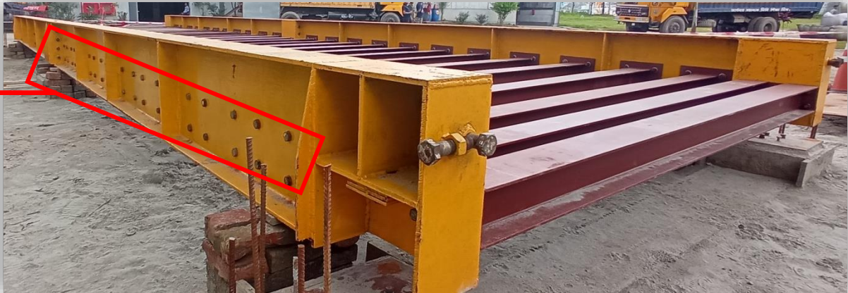
Picture: GATCOBD Truck Scale Nut-Bolted System
