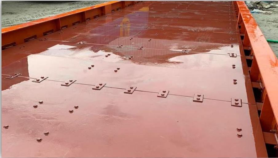
Picture: Nut-bolt System in GATCOBD Truck Scale
